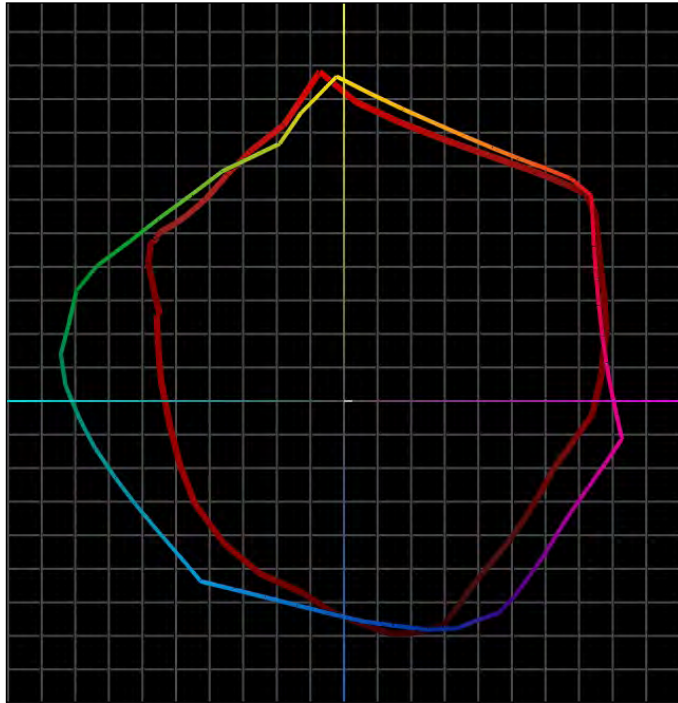
Epson SureColor T3000 24" colour gamut on photo quality paper in Max Quality settings (red) versus Canon imagePROGRAF iPF680 colour gamut (shown chromatically) on photo quality paper in High quality settings.
