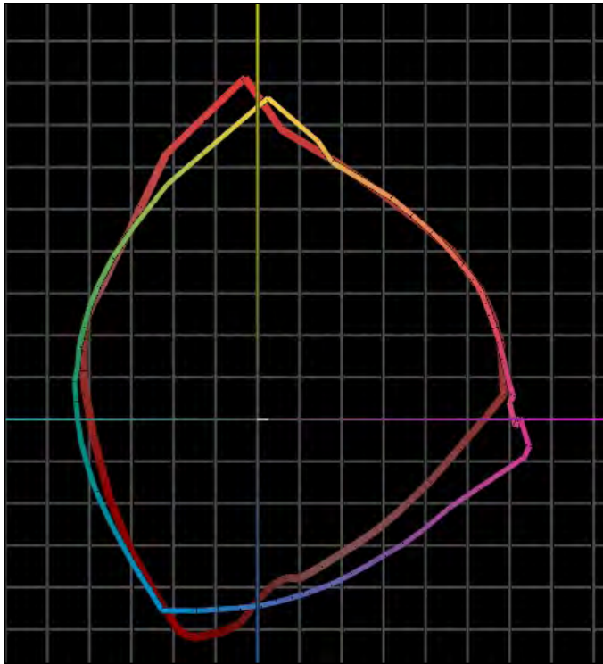
Epson SureColor T3000 24" colour gamut on plain paper in Max Quality settings (red) versus Canon imagePROGRAF iPF680 colour gamut (shown chromatically) on plain paper in High quality settings.
