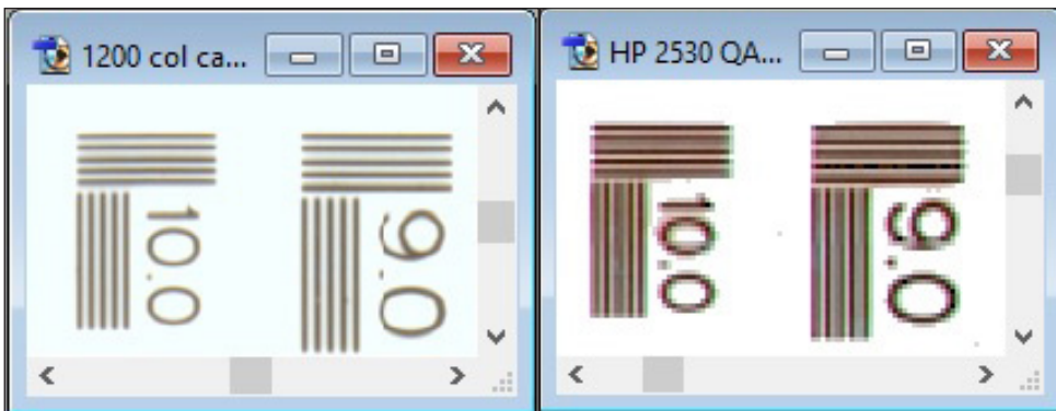
Canon (left) and HP (right) fine line pairs at maximum resolution. The Canon lines are much more distinct.
