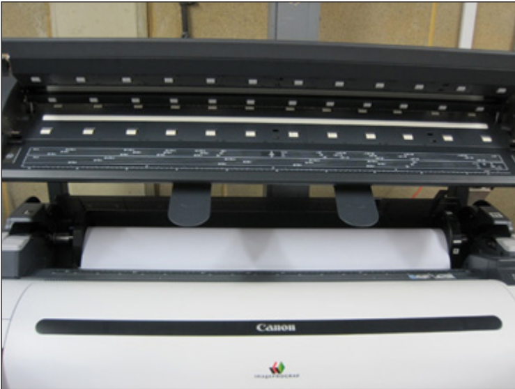
Canon's SingleSensor array extends across the full width of the scanner.
